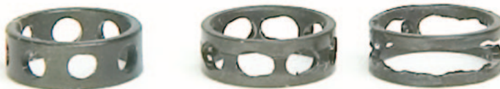
A bearing retainer is shown here in three stages of its life—new (left), worn (center), and catastrophic failure (right).
